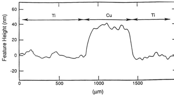
The Profilimeter trace above comes from the class and shows dishing of the titanium liner relative to the adjacent recessed copper metal. An electrochemical interaction between the copper metal and the titanium accelerated the normally low polish rate of titanium to produce the negative dishing.
